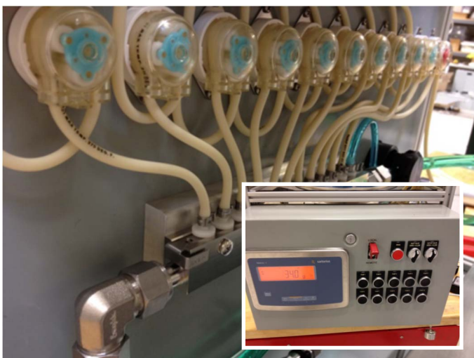
Crud sampling system and control unit
