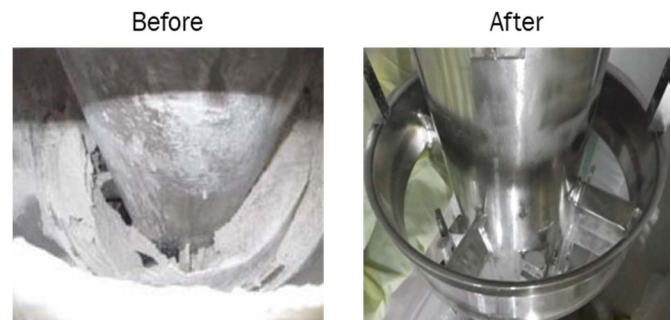
NU-DEC™ cleaning results (radwaste cement solidification system vessel)
