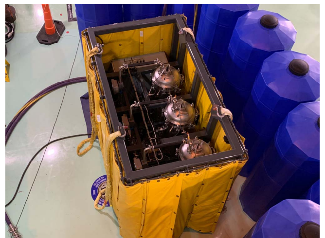
AMFM-S300 filter system used during cleaning
