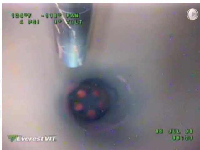
Insertion of transducer into BWR jet pump
